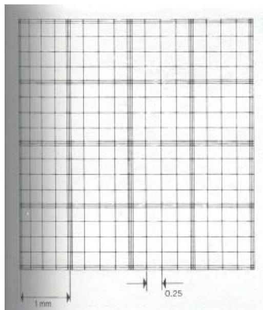
**1158 COUNTING CHAMBER, NEUBAUER, modified model, depth 0.1 mm**
