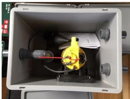
**5157a Submersible electric dirt water pump, 230V, with adapter to fit 1" male thread**
